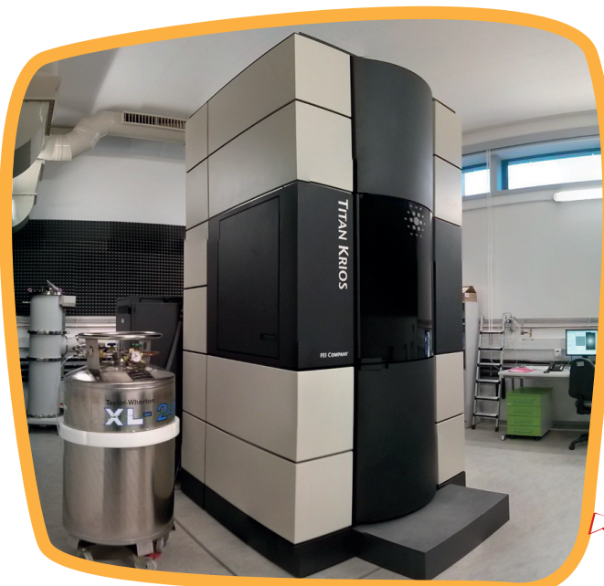
Electron microscope Titan Krios enables imaging of biological macromolecules embedded in vitreous ice.
